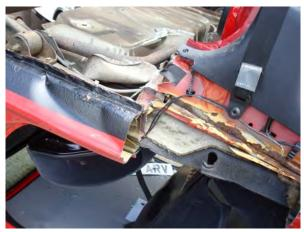
Here you can see we have completed all the cuts with a reciprocating saw as the sill was very weak with the age of the vehicle.
