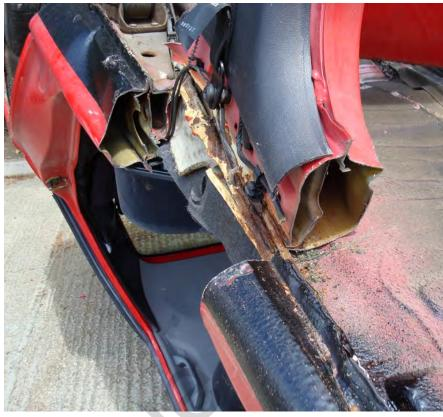
What is also important to look for is additional strengthening in the Sill / rocker channel, as sometimes in newer vehicles we will find a circular strengthening tube that we may not be able to cut through with old cutters or recip saws this will only be visible once you have cut through the outer skin.
