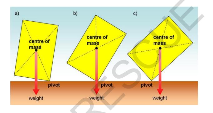
These are all factors that a rescue team should take into account during a rescue, in cases where the vehicle is not on all four wheels and is precariously positioned, good stability needs to be put into place to create a safe working environment.
