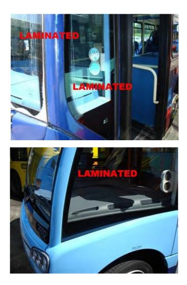
Passenger side windows will be toughened glass and can be dealt with in the same way we do cars, with a center punch and so on.
