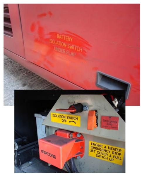
If you still feel that the battery cables need to be disconnected, you can access the batteries from the front or side of the bus. A budget key or screwdriver will normally open the locker where the batteries are kept. Only one set of terminals needs to be disconnected.
