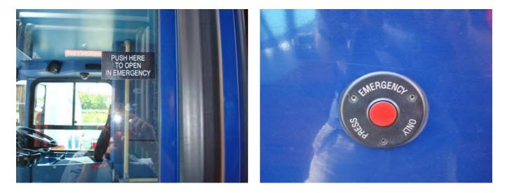
If the system has air in it, you can just push the emergency door release button. However with the door system charged with air there will be a need to secure the door open as it will try and self close.
