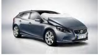
This type of protection developed by Volvo isn't far from hitting the roads. At this time we need to be aware of its presence especially during a vehicle fire as a projectile hazard, or during forced battery access.
