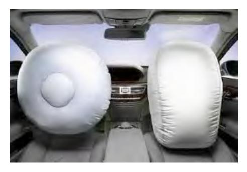
Frontal airbags come in many different sizes and shapes, these are ever changing due to new technology and vehicle crash testing, however for the rescuer this poses a headache or does it?
