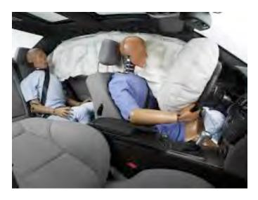
Side airbags will in most cases only deploy from side impacts, however with new vehicles and SMART systems analyzing the crash data it may now be found that these systems may also actuate in a frontal collision, don't forget there may be other forces such as rotational force from rebounds etc.
