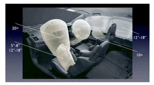
\*Due to the ongoing developments in airbag size and shape, the distances - 5, 10, 15, 20 are no longer a reliable guide, use them for reference if needed. These have been replaced with the control of "AVOID DEPLOYMENT PATHS"\*
