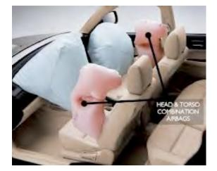
This type of airbag is also a one time activation, once deployed they are safe to work around, these can either be deployed form the B-post, seat or fitted into the door, so a thorough scan for these airbags needs to be carried out.
